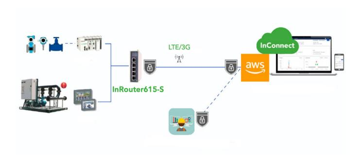
PLCs, HMIs and other smart devices around the well and compressor sites are connected to the IR615-S via Ethernet ports. Data collected from the now connected devices are then securely sent (encrypted) via OpenVPN, to the InConnect VPN platform via the LTE cellular networks, so that engineers can monitor these devices anytime from anywhere.
